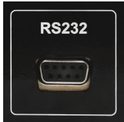
Fig. 10: RS232 controller connector
