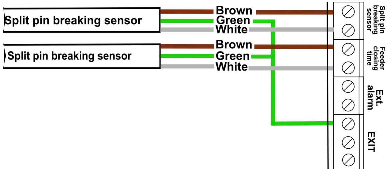
Picture 3: Connecting the sensors of split pin breaking and of closing the storage unit.
