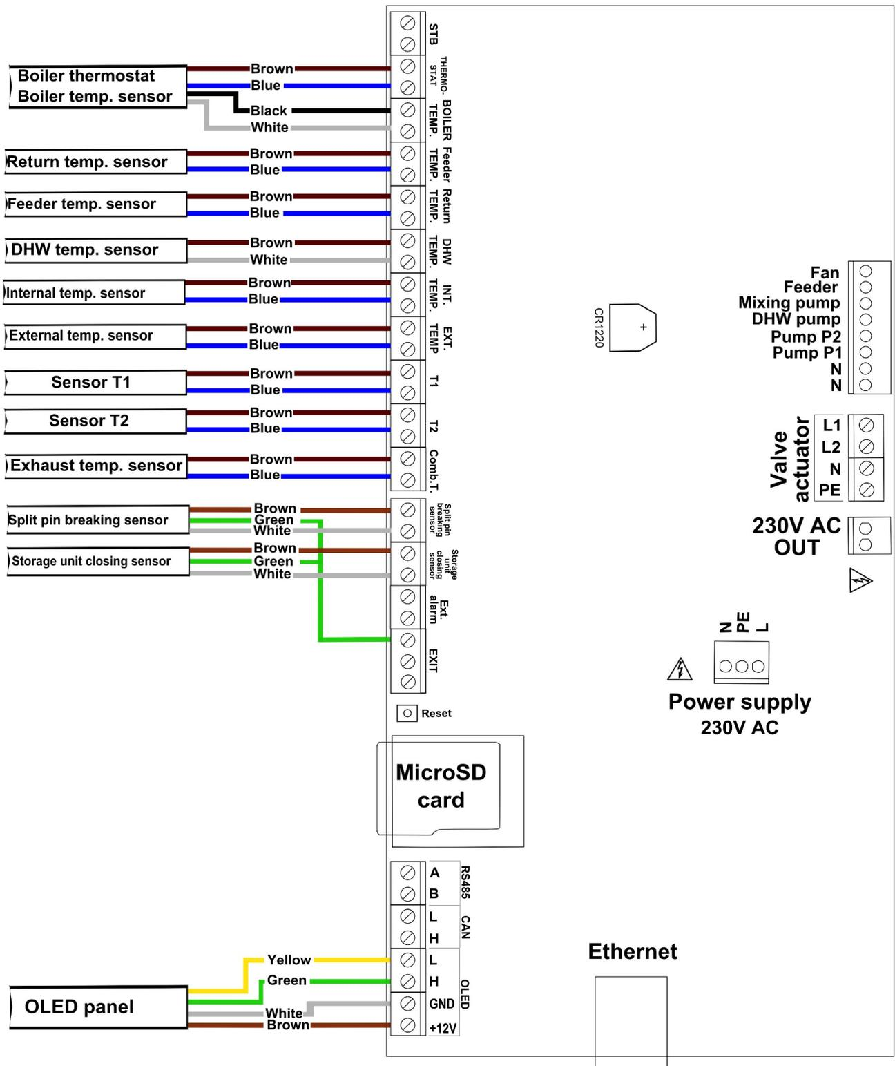
Picture 2: Terminal strip for connecting the sensors
